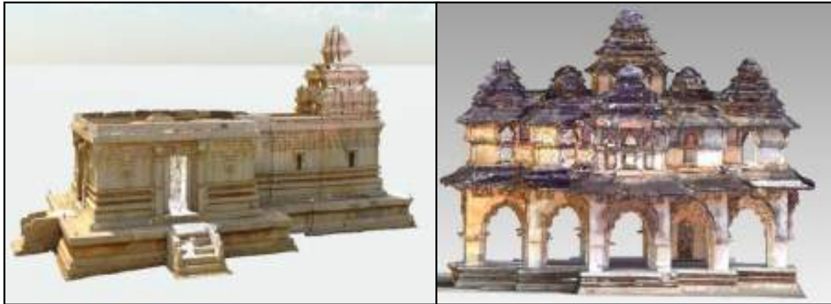
3D Point cloud data of Balakrishna Temple and Lotus Mahal in Hampi
