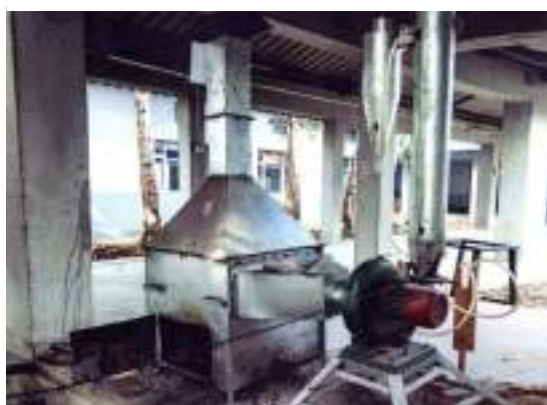
“A fluidized bed paddy dryer with waste heat recovery suitable for NER, India” by Dr. Pankaj Kalita
