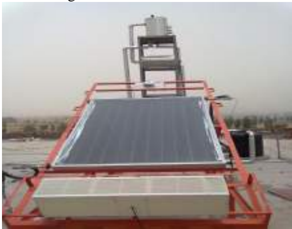
Thermal Performance Test Set-up
