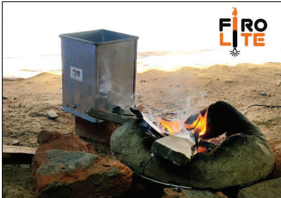
“Design & Development of a portable thermo-electric generator, FiroLite” by Kaustov Gopal Goswami, Guwahati
