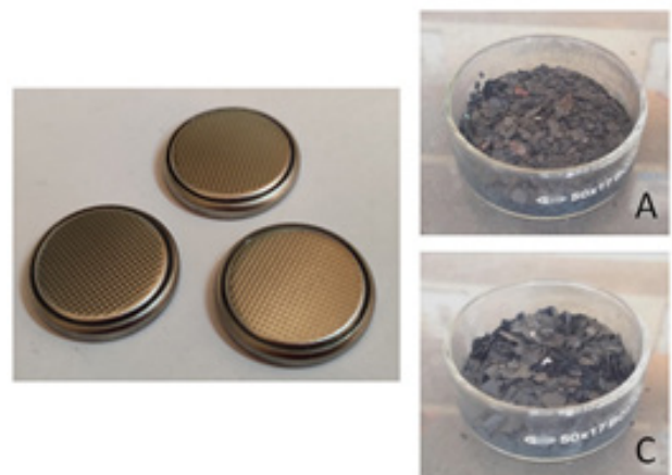
Coin cells fabricated from recycled anode (A) and cathode (C) material
