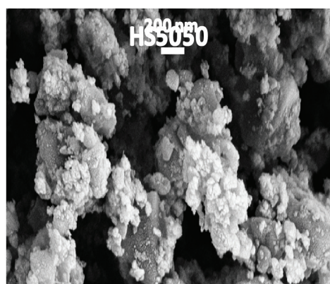
SEM image of high capacity hard carbon-anti-mony composite
