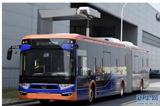
A new electric bus based on supercapacitor technology was put into operation in China in 2015. It is capable of achieving full charge in 10 seconds.
