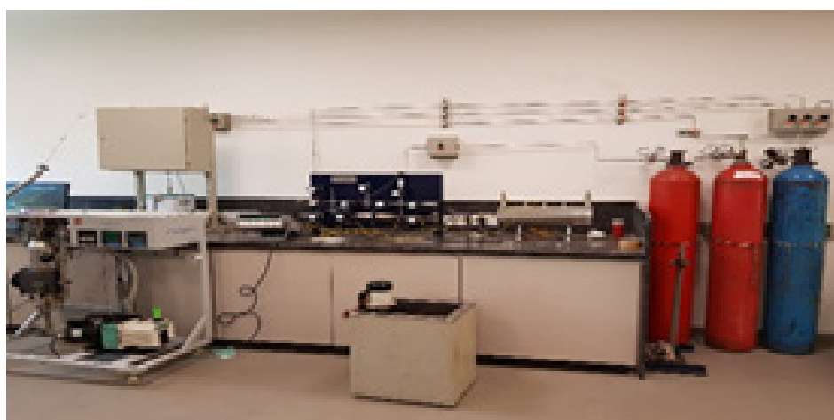
Measurement setups (Static & Dynamic PCI Indigenously developed)
