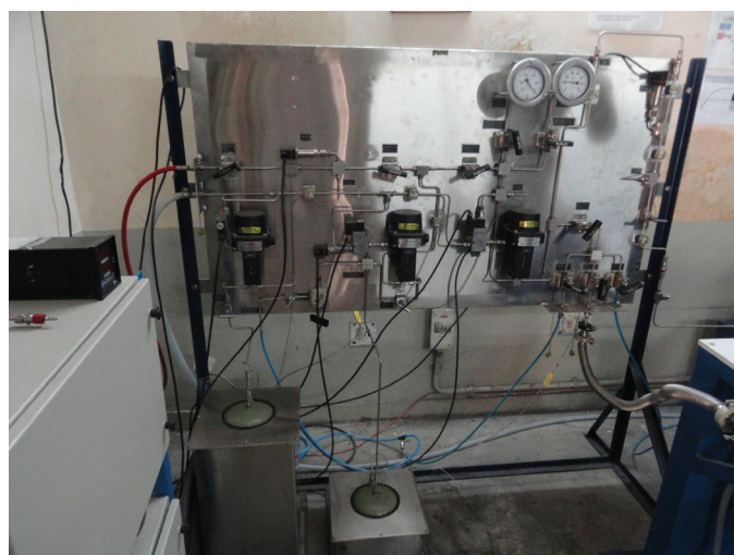
PCT apparatus developed at NFTDC – Supplied to IIT M
