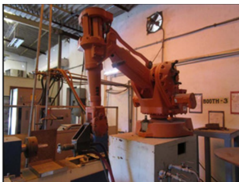
Plasma Lab at NFTDC for spray coating for Fuel Cells
