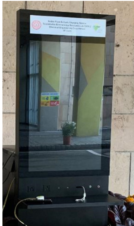
Fig. Flow battery based charging station developed by SERL, Department of Chemical Engineering, IIT Delhi
