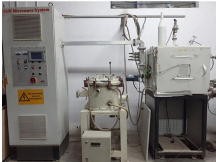
6 kW microwave set up for producing Graphene - NFTDC
