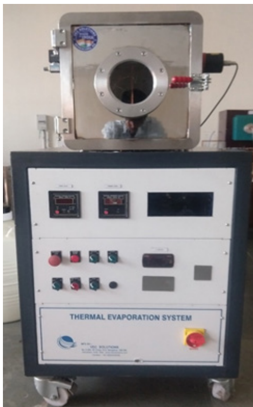
Thermal evaporation system
