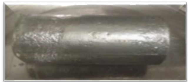
Casted alloy from Vacuum Centrifugal Caster
