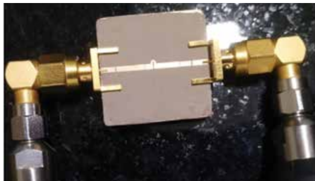
Omega resonator for NV center fabricated at IISER Kolkata.
