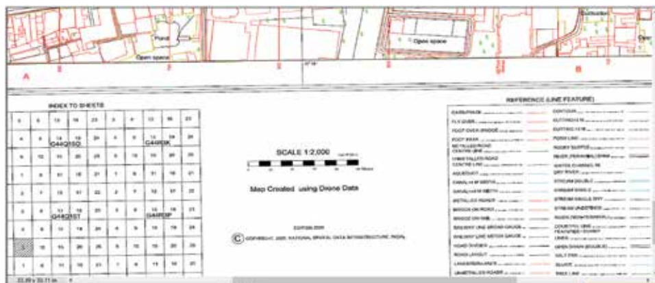
(Figure 4: Focus on Data Life Cycle Management - Display of a part of an up-to-date 1:2,000 scale National Urban Information System topographic map of Varanasi City prepared using drone surveys conducted during October - November 2020. Local level network of high-resolution topographic grids with index numbers consistent with the National Topographic Frame for monitoring drone-based surveys has been shown)
