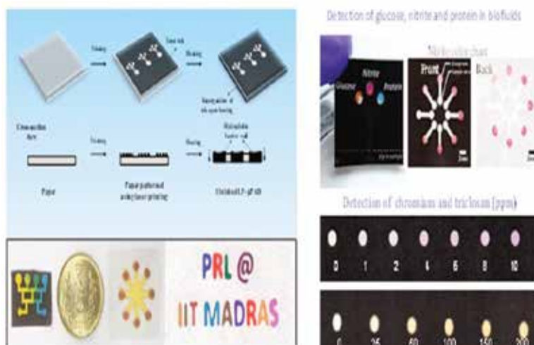
Figure 7. A novel microPAD fabrication method and device development method
