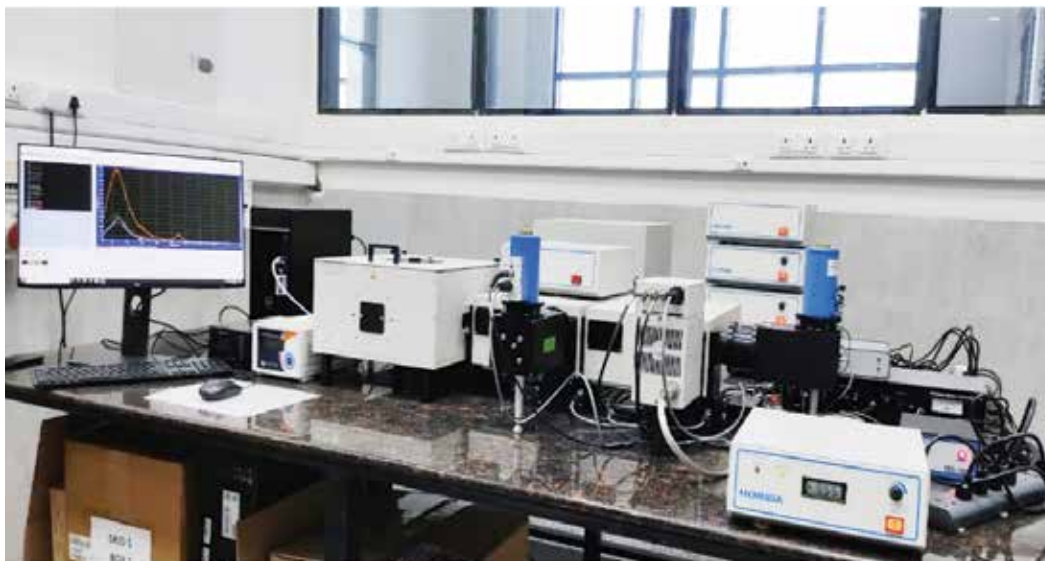
State-of-the art Steady-state photoluminescence (PL) spectroscopy facility of SATHI at Sonipat Campus of Indian Institute of Technology Delhi
