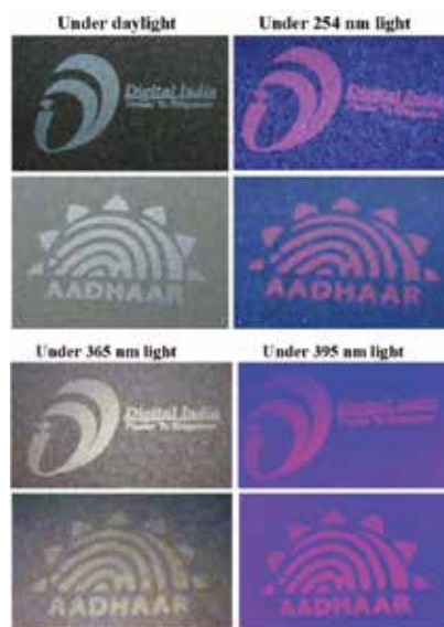
Digital images of Digital India and Aadhaar logs printed with security ink on black paper under daylight(white), 254(red), 365(greenish yellow), and 394 nm(pink) UV light.
