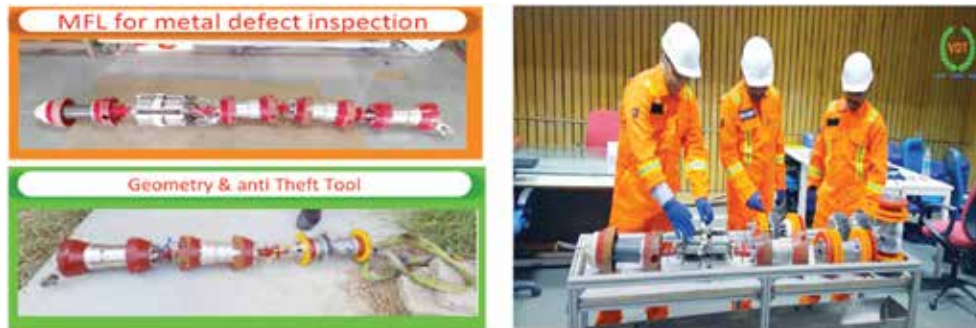
Fig 5. VDT pipeline integrity tools
