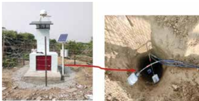
Figure 3. GPS-Soil Moisture Observatory at JNV, Aurangabad, Bihar (Left). Three Digital Hydra Probe soil sensors installed at three distinct soil horizons (Right).
