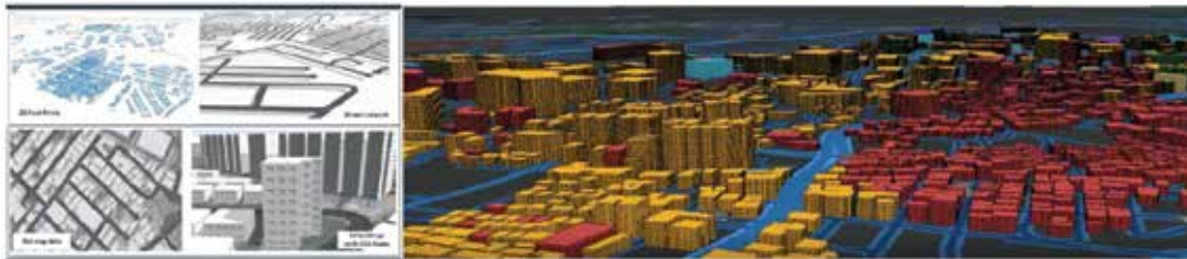
Figure 6(a): 3D Modeling of LOD 2 buildings extracted from generated building height Models
