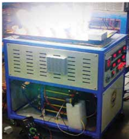
(Integrated 1kW Polymer Electrolyte Membrane Fuel Cell System with power conditioner for plugin type AC application)
