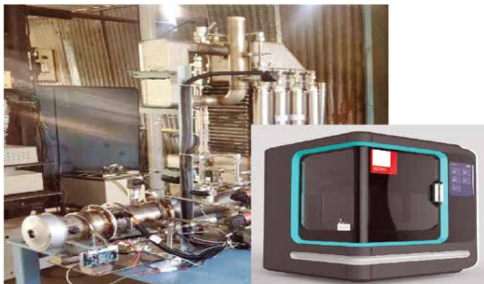
Figure 1. Methanol fuel processor and methanol powered high temperature polymer electrolyte membrane fuel cell system prototype
