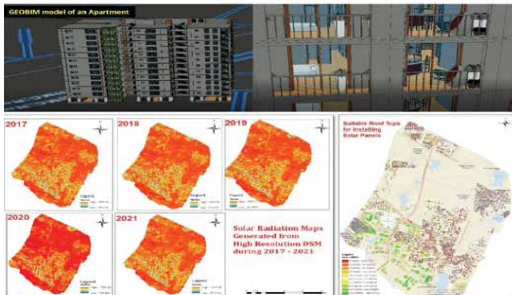
Figure 6(b): Geo BIM Model and Roof Top Suitability analysis for installing Solar panels
