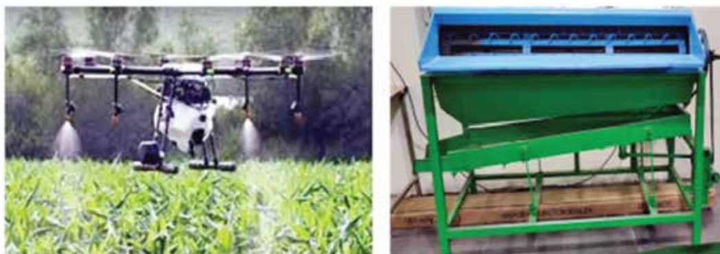
Fig 8. Smart Agro Sprayer & Dual Mode Groundnut Pod Stripper developed
