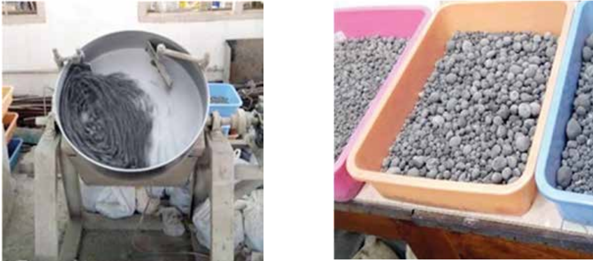
Fig: Laboratory trial production of Geopolymerized Aggregates
