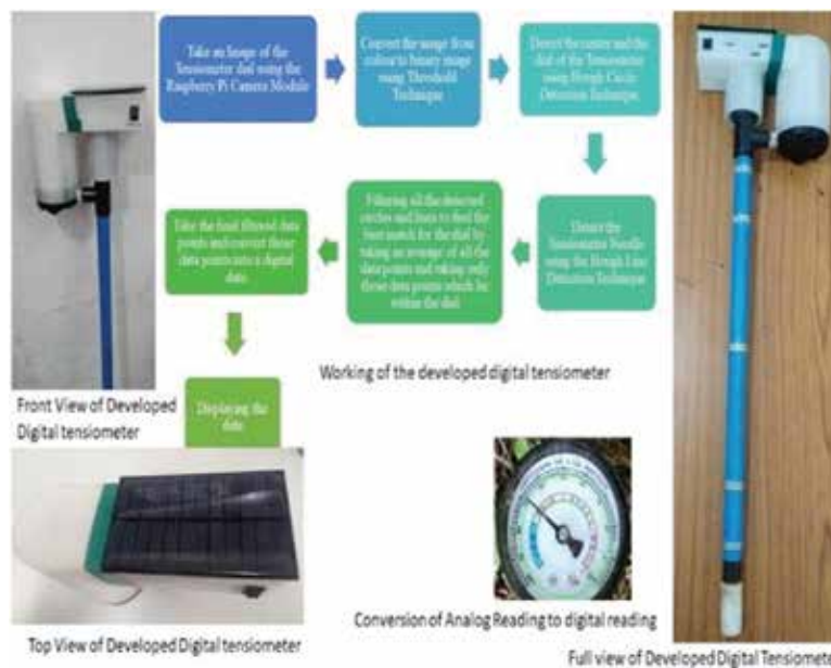
Fig.1. Digital Tensiometer based on Image Processing
