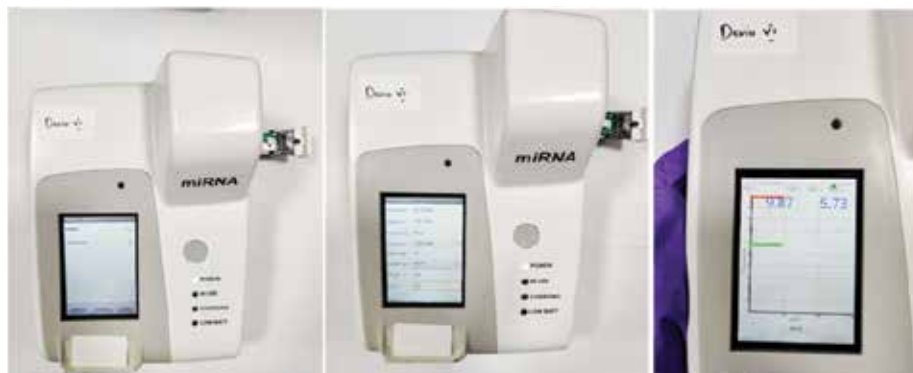
Figure shows the instrument developed and the process for measuring the miRNA level, a. the initialization to choose calibration or miRNA measure, b. Patient details entry, c. the result. The instrument has 2 channels to display the miRNA levels of miRNA 21 (Over expressed) and miRNA 195 (suppressed).
