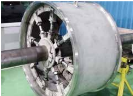
Fig. 2: Vacuum vessels under fabrication (INOX India, Vadodara)
