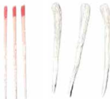
GP coated with AFPG glass granules & with Ag Nanoparticles
