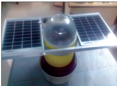
Photo Voltaic integrated Surya Jyoti
