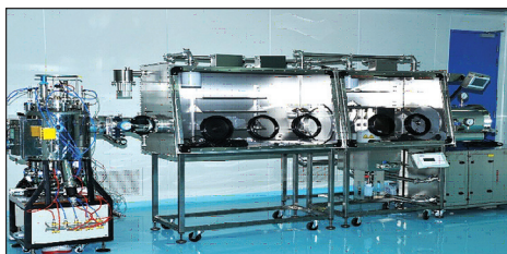
Inert glove box based organic solar cell device fabrication facility created under INDO-UK Solar Energy
