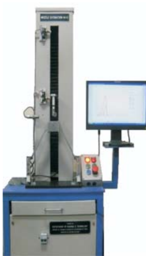
Fig. 4.11: Instrument for measurement of fabric feel by nozzle extraction developed at IIT, Delhi
