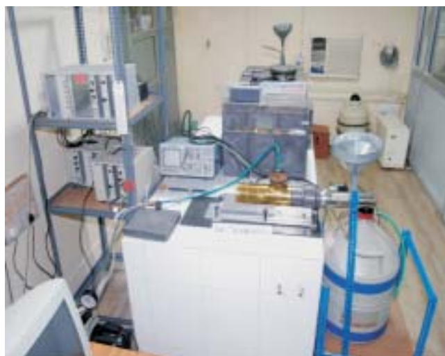
Fig. 1.22. First-Indian 20 Ci Cs and first-ever shortest geometry 100 mCi Am Compton spectrometers developed by group of Prof. B.L. Ahuja, M.L. Sukhadia University, Udaipur (Rajasthan)
