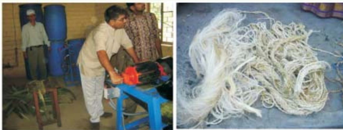
Fig. 5.7: Multi-Fibre Extraction Machine Prototype & Mechanically extracted Fibres of Grewia optiva
