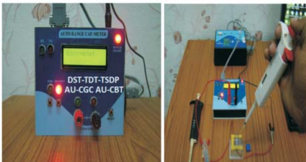
Fig. 4.48: Portable auto-range capacitance meter for reagent less measurement of enzymatic reactions ( left : capacitance meter ; right : Measurement set-up with reaction cuvette)
