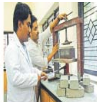
Fig 5.10: Making of bricks using hand operated machine
