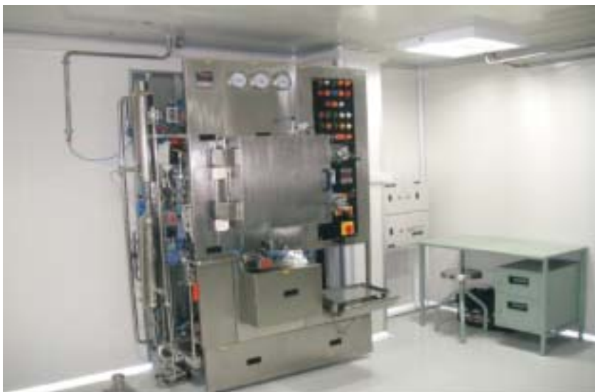
Fig. 4.1: Close up View of PLC-Controlled Autoclave at BSL-3, IISc, Bangalore
