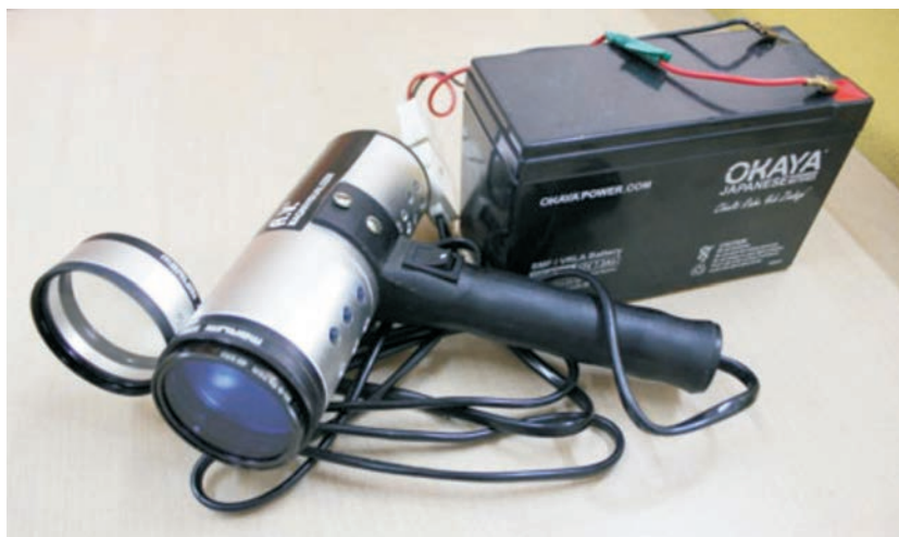
AV Magnivisualizer, equipped to work on a 12-volt portable rechargeable battery
