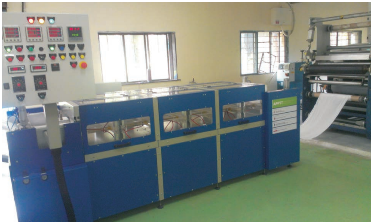
Plasma reactor developed by FCIPT, IPR and functioning at MANTRA, Surat
