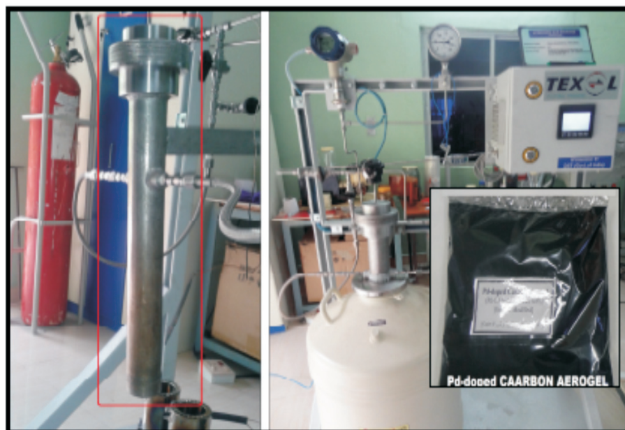
Prototype device for storage of H 2 in carbon aerogel ( in-set : Pd-doped carbon aerogel)
