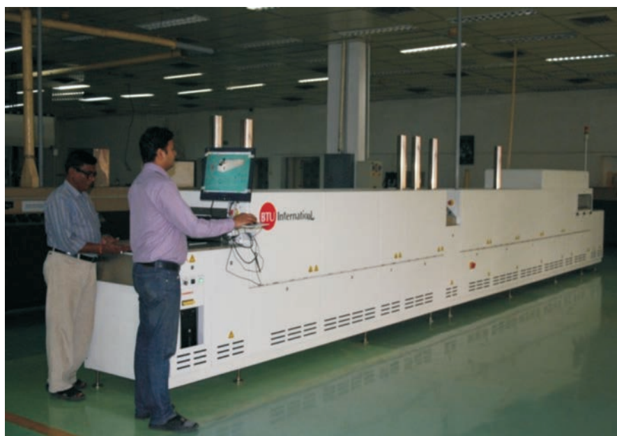
Dryer cum firing furnace
