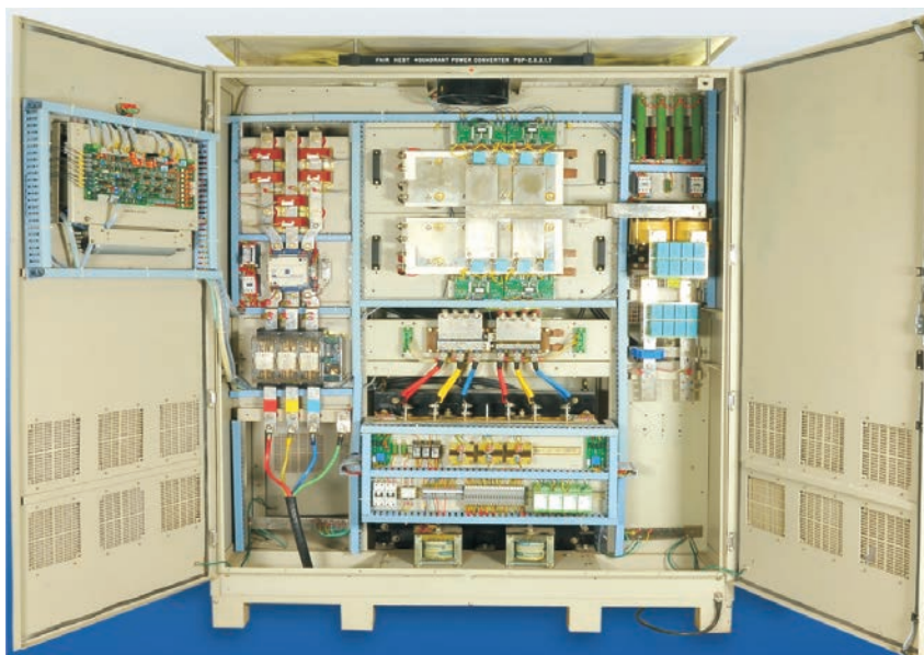
Fig. 1: A Prototype of Power Converter built at ECIL
