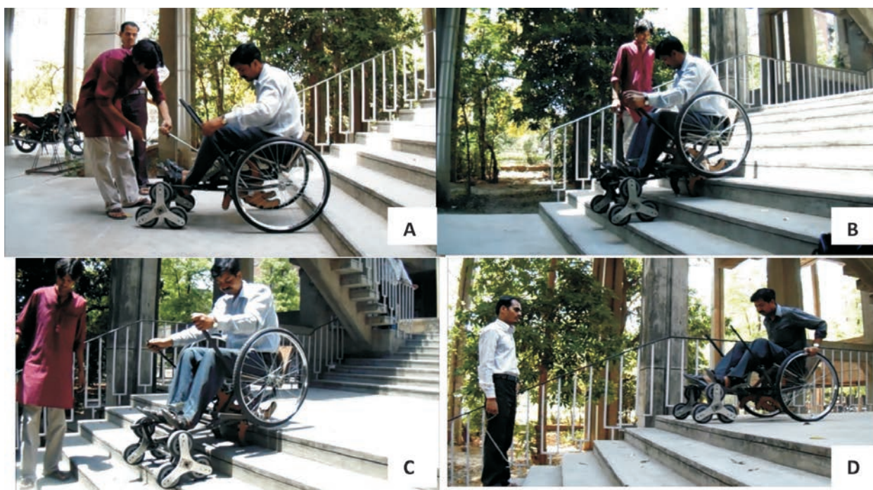
Figure A, B, C, D describing sequence of convertible mechanism from flat floor to stairs and then from stairs to flat landing space
