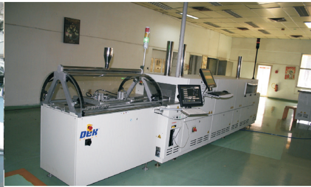
Screen printer and curing furnace for special paste (BHEL)
