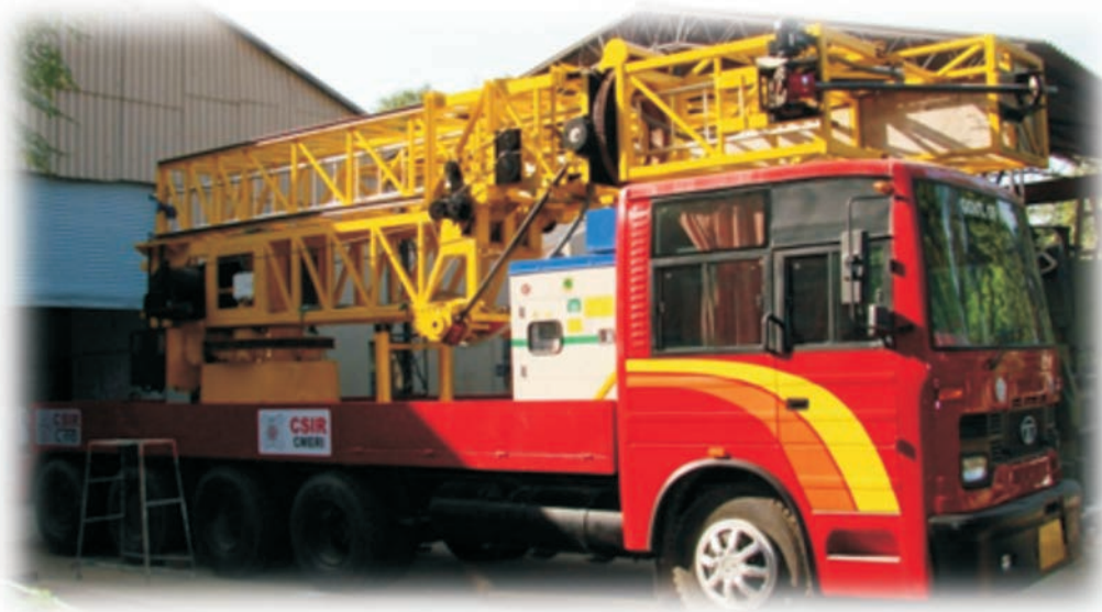
Mobile Bridge Inspection Unit (MBIU)
