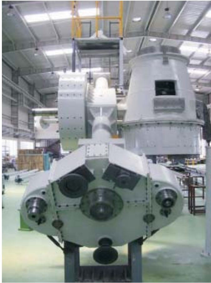
Assembly and testing of 50-cm B-N Schmidt telescope at M/s Pedvak, Hyderabad.
