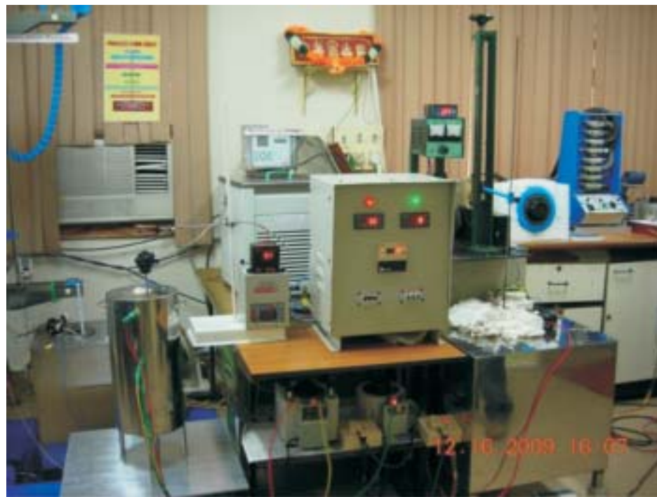
Novel Plasma Reactor for production of Nano Alumina at Dalmia Institute of Scientific and Industrial Research, Rajgangpur, Orissa
