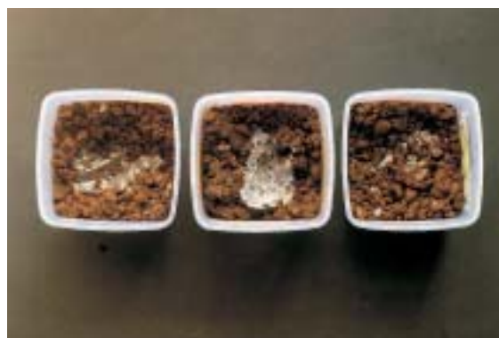
Biodegradability testing of PHA film formed by Halomonas sp. by soil burial method in soil containing 25% moisture. Intact PHA film (Left), PHA film degraded after 1 month (Centre), PHA film degraded after 2 months (Right)
