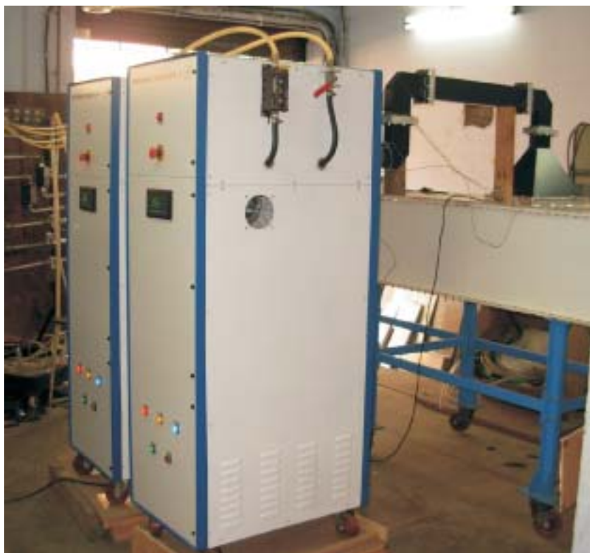
Variable power 10 kW Microwave System developed for Tea Drying has successfully been installed at tea garden of M/s Koomtai Tea Estates, Assam
