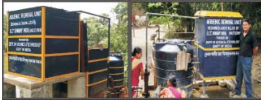
Arsenic Removal Unit in West Bengal
