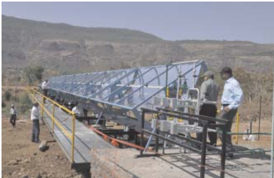
Fig. 4.47: Pilot Testing of Parabolic Troughs at Shive Village, Pune
