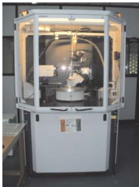
Fig. 2.5: Single Crystal X-ray Diffractometer at the S
