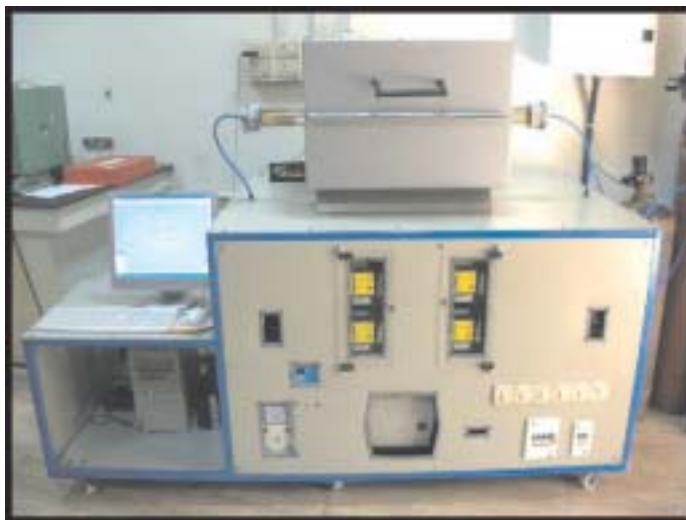
Fig. 7.13: Automated experimental facility for CVD process (10 g of CNTs in a single step)
