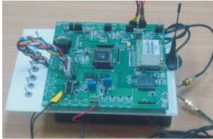
Fig. 5.24: Low cost general purpose wireless sensor node for deployment in the IITB Smart Campus Grid Project for the management of campus resources
