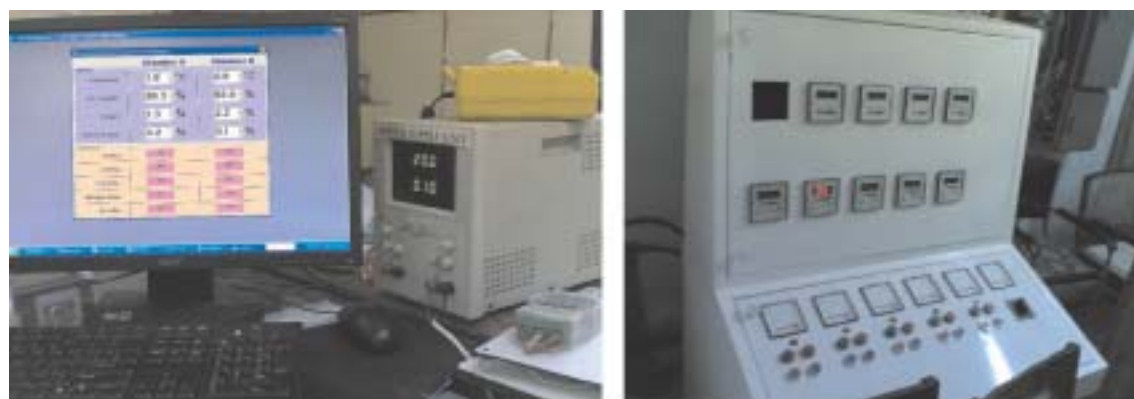
Fig. 4.4 : Computerized Control System for CA stores
