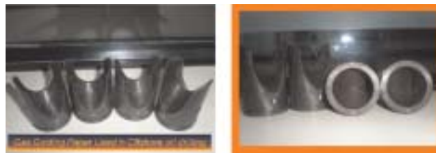
Fig. 4.36: Gas guiding paper used in Off-shore Oil Drilling (PP/Banana/Glass Hybrid composites)
