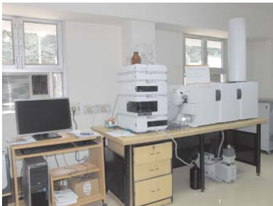
Fig. 2.3: Q-TOF High Resolution Mass Spectrometer at the SAIF, Lucknow
