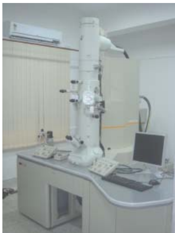
Fig. 2.4: 200 KeV Transmission Electron Microscope at the SAIF, Shillong
