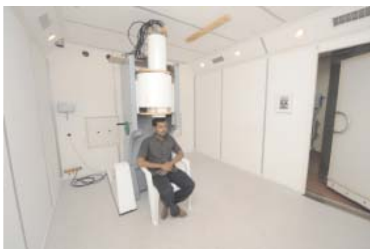
Fig. 2.6: MEG system inside the Magnetically Shielded Room.
