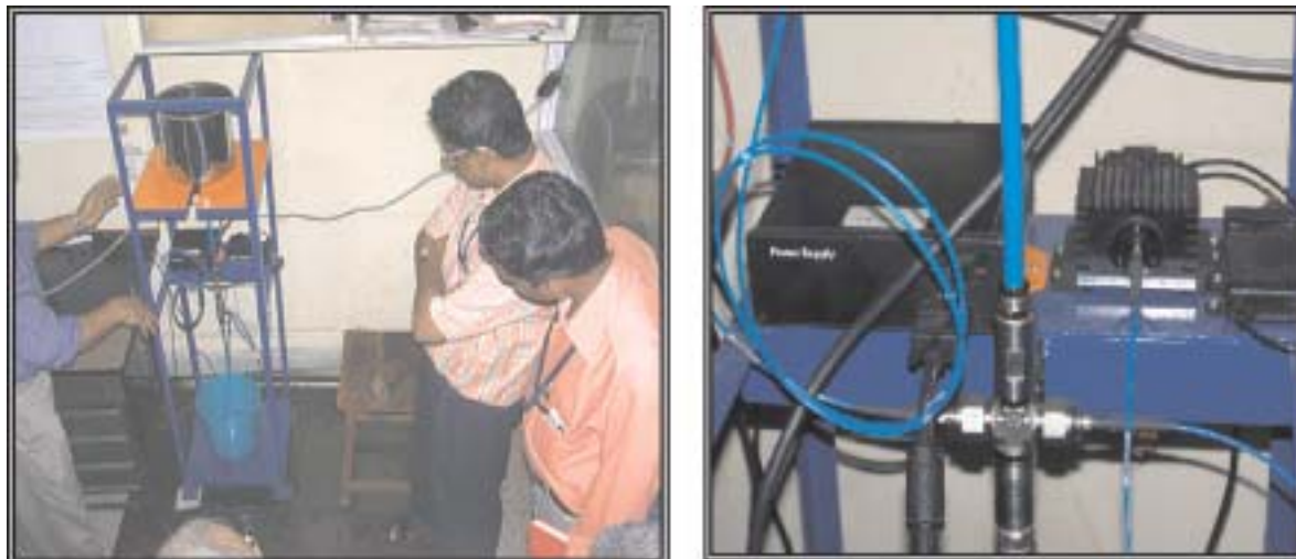
Fig. 4.11 : Near Infra red spectroscopy based on-line instrument
