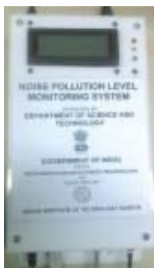
Fig. 4.6 : Noise pollution level monitoring system for textile industry
