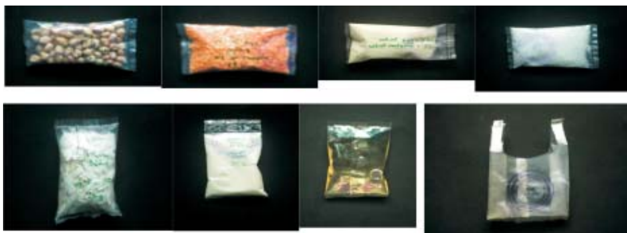
Fig. 10.2: Polymer bags prepared using PHA films formed by Halomonas campisalis
