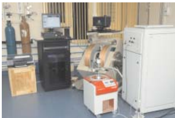
Fig. 2.1: Vibrating Sample Magnetometer at the SAIF, Chennai.
