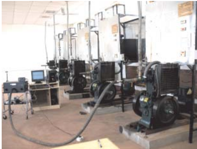
Fig. 4.39: Experimental test set up (5 nos) for single cylinder IDI diesel engine (Test fuels: Diesel, JSVO10, JSVO20, JSVO50 and neat Jatropha oil at University of Petroleum and Energy Studies, Dehradun)
