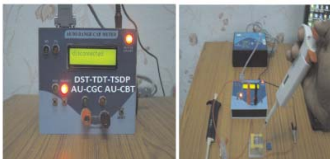
Fig. 4.41: Portable auto-range capacitance meter for reagent less measurement of enzymatic reactions (left : capacitance meter ; right : Measurement set-up with reaction cuvette)
