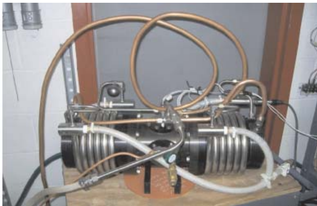
Fig. 1.32: Valved Oil free two stage Linear Motor compressor
