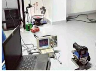
Lab set-up: The paint on the speaker is being excited at definite frequency and a slow-motion camera films the jets as they form. • O.V.S.N. MURTHY
